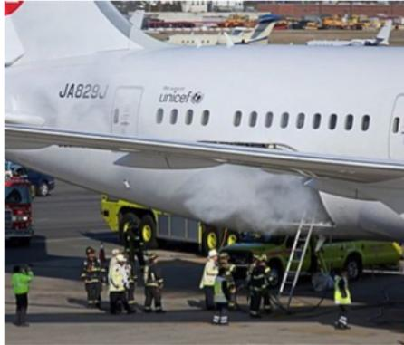
The incident resulted from **Boeing's failure to incorporate design requirements** to mitigate the most severe effects of an internal short circuit within an APU battery cell and the **Federal Aviation Administration's failure to identify this design deficiency** during the type design certification process
